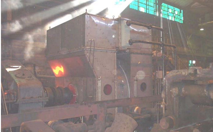
Picture 4 - Final design with air-to-water heat exchanger
