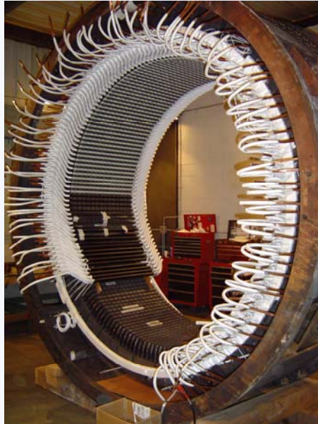
VA Tech Hydro unit during rewind.
