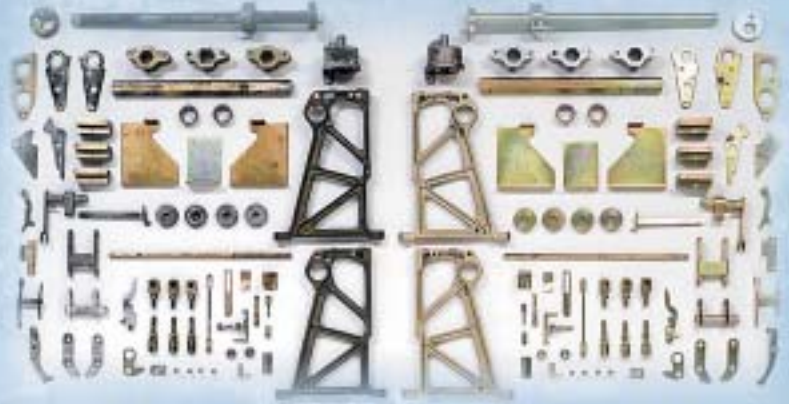
ITE KD circuit breaker after refurbishment.
