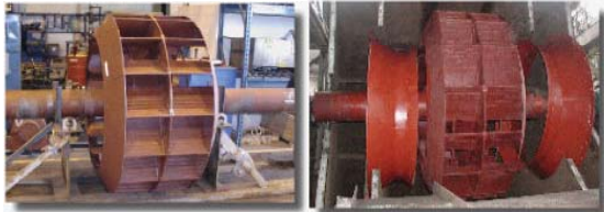
Turnkey rotor removal/installation completed in 30 hrs.
